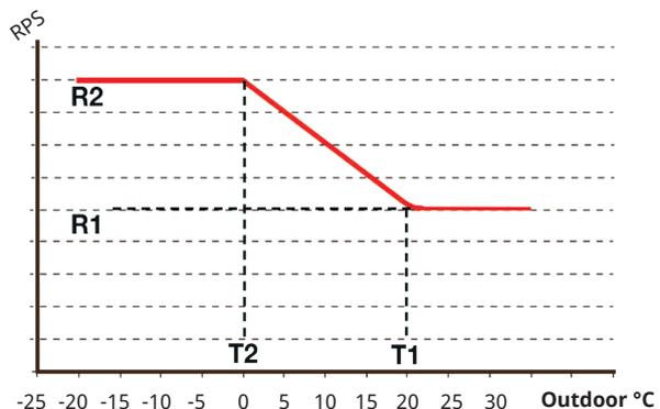
The diagram shows that the compressor speed is controlled according to the outdoor temperature.
